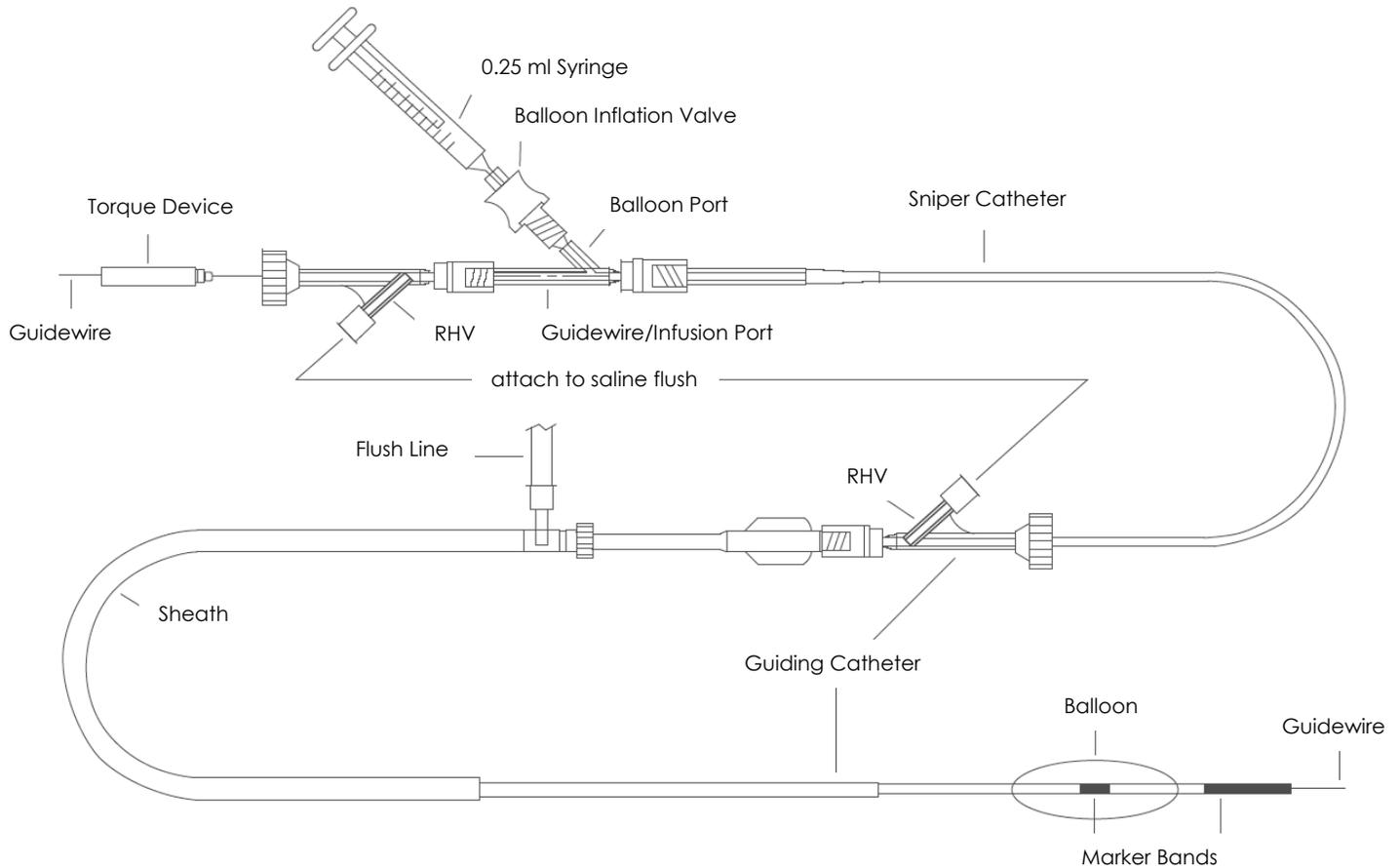
**Figure 2:** Procedural Setup and Configuration
